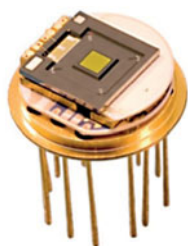
MEMS based micro spectrometer module and spectral response (from InfraTec)
