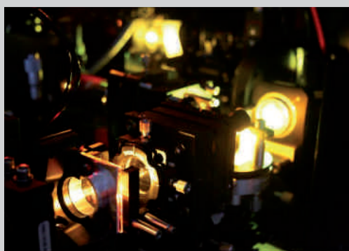
Interferometric setup to measure the complex transmission response of complex metamaterials.
