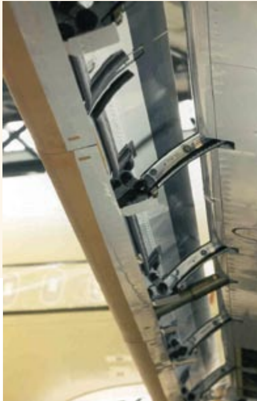
Wing with extended slat tracks during MRO. The transition from time-based to condition-based maintenance, based on Lamb wave ultrasonic inspection, will be the focus of AISHA.
