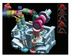
**Figure 1.4** The variable valve actuation (VVA) system, controlling lift and timing of the engine valve by means of an electro-hydraulic system, enabled new combustion strategies of the gasoline engine.
