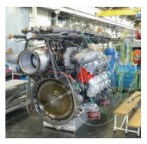
Figure 4.1 MTU (series 4000) V8 engine at the test bench and a typical locomotive application.
