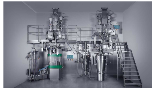
ConsiGma 25 (GEA) + Courtoy tablet press for continuous processing – exemplary layout Source: GEA, www.gea.com
